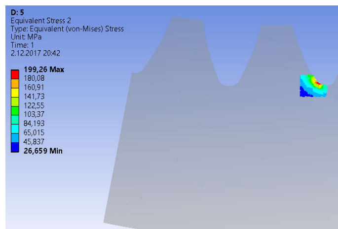
Figure 7. Bending stress result for 0.2-0.2xm tip radius and 5xm rim thickness
