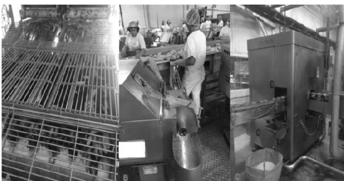
Figure 2. Photo of a plunger (A), corn stripper (B), and sealing machine (C) in the company studied
