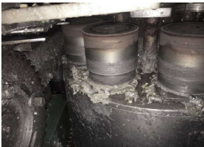
Figure 6. Lack of adhesion of the grease on the harvester
