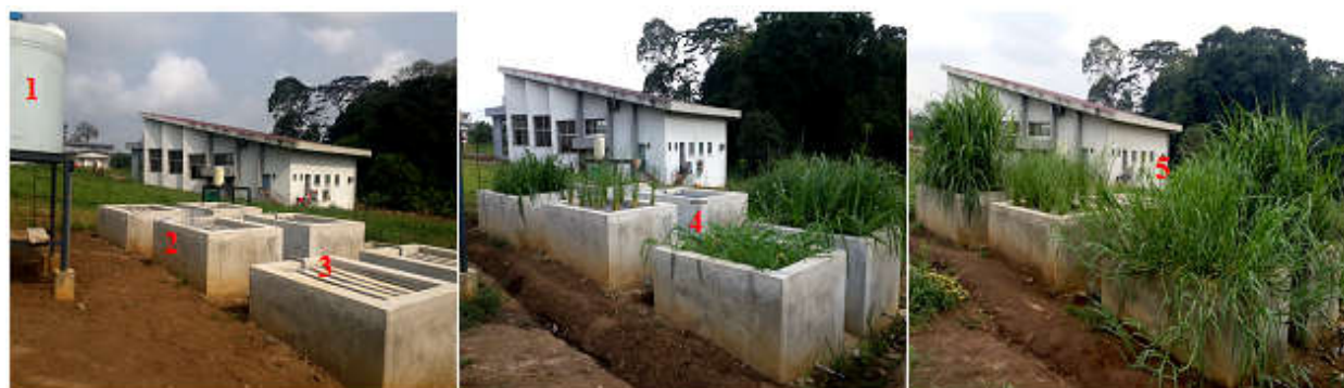
Fig. 1. View of the experimental wetland system, 1: feeding tank, 2: bed, 3: irrigation device, 4: plants growing on the beds after one month and 5: plants growing on the beds after two months
