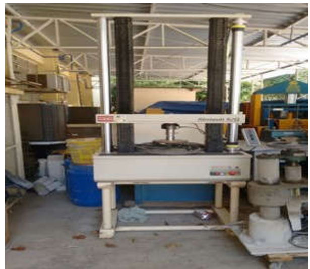
Fig. 7. Equipment Sintech 5/G for traction resistance test
