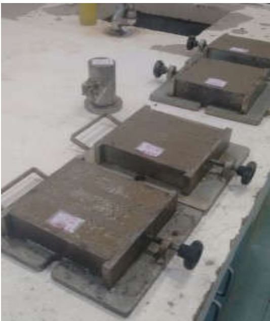
Fig. 3. Specimen molded with mortar
