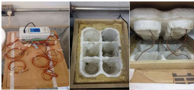
Fig. 5. Equipment FieldLogger, to the left with the cap closed, in the middle with the cap open, where the mortar was placed for the data collecting and, to the right, with the mortar inserted in equipment
