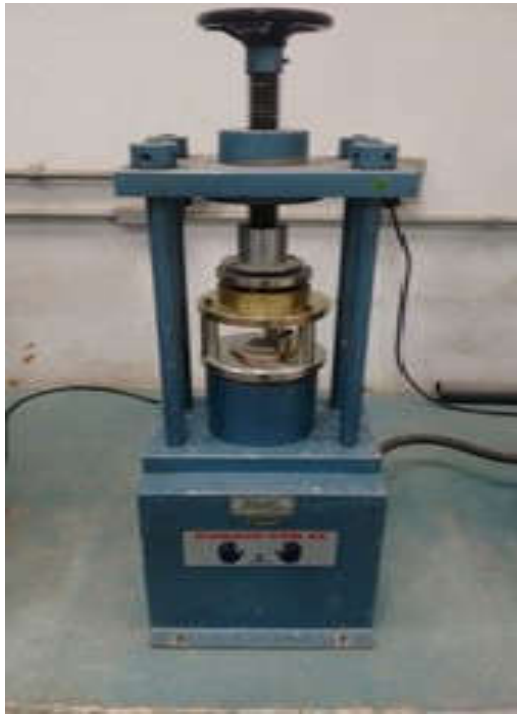
Fig. 9. Equipment Sintech 5/G for realization compression resistance test
