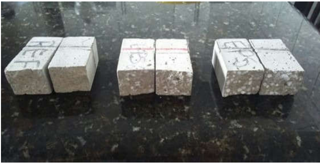
Fig. 13. Specimen broken after compression test at day seventh. From left to right: reference marks, displacement marks with 20% and displacement marks 40%, respectively
