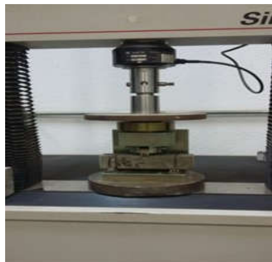
Fig. 8. Test of resistance to the bending traction with equipment Sintech 5/G with specimens at 7th day
