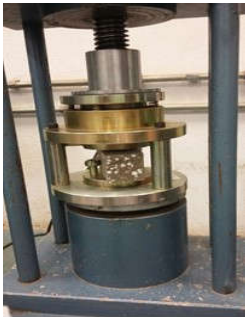
Fig. 10. Resistance to the tension in the compression test, with equipment Sintech 5/G with specimen of seven days
