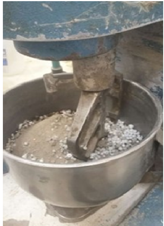
Fig. 1. Preparation of mortar in mechanical mixer
