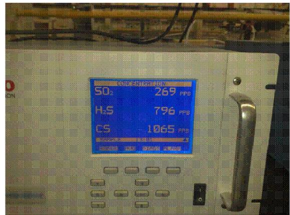
Figure 3. Thermo Electron Corporation 450i H<sub>2</sub>S/SO<sub>2</sub> gases analyzer
