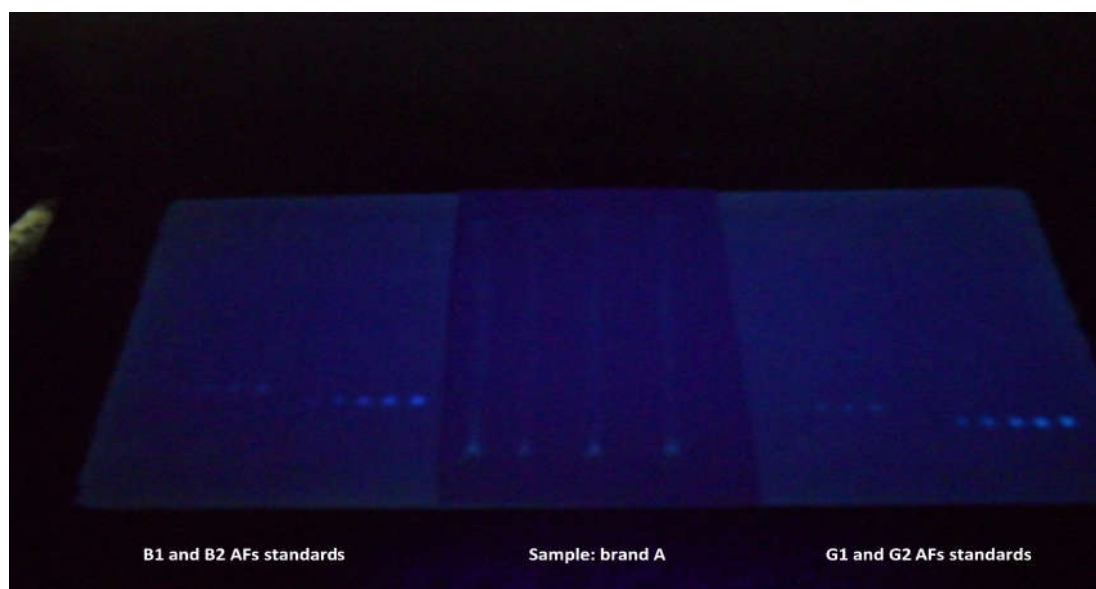
Figure 1. TLC analysis of the peanut butter candy brand A under Ultra-violet light. From left to right the application was: Aflatoxin standard B1 and B2; Sample; Aflatoxin standard G1 and G2
