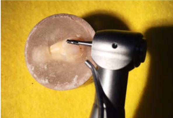
**Figure 4. Removal of the remaining resin with multilaminated drill**
