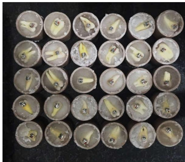
Figure 2. Test specimens with their respective brackets adhered
