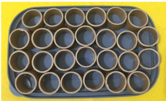
Figure 1. Plastic cylinders with 25mm in diameter and 20mm in height
