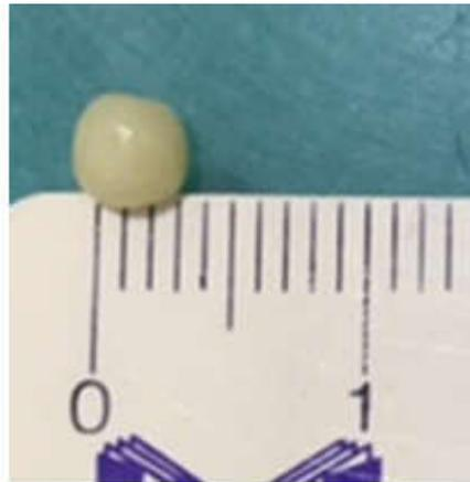
**Figures 5 e 6. Resin increase of 3mm measured on the ruler and applied to the specimens**
