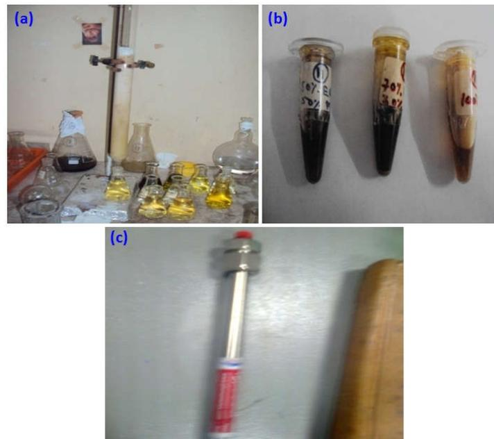
Fig. 1. (a to c) (a) Column chromatography extractions, (b) Concentrated solvent extracts with different concentrations, (C) PLC column: (Bio Sep - SEC- s2000)
