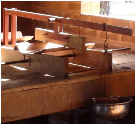
Figure 1. Device of resistance tests in the flexion.
