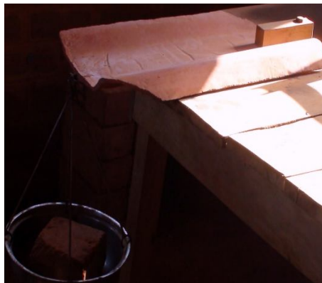
Figure 3. Device of resistance tests in the drive of the heel.
