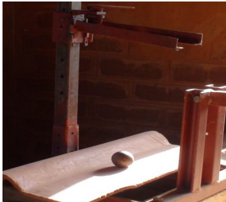
Figure 1. Device of resistance tests in the flexion.
